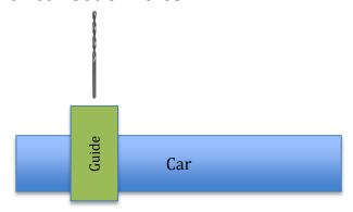
Keep the Drill bit perpendicular to the car body and guide.
